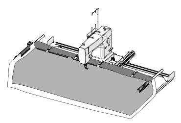
2 Press the coil clamps onto the front rail to hold the fabric in place. Make sure that the **end of the coil that is attached** to the clamp is on the inside of the frame. **Note:** The front clamps work best when attached from the front of the front rail, rather than from the top of the rail.
