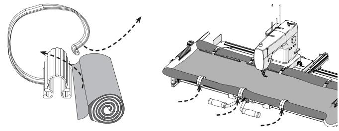
4 When it's time to move your fabric, remove the fabric roll from the coils. To remove the fabric clamps from the front rail, pry the lips of the clamp away from each other and then pull the clamp off the rail.
