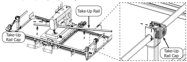
If you're using the coil clamps on the **front rail**, then remove the front rail from the frame by raising the two **side rail levers** on the sides of the frame, and sliding out the front and side rails. <u>Otherwise</u>, skip this step.
