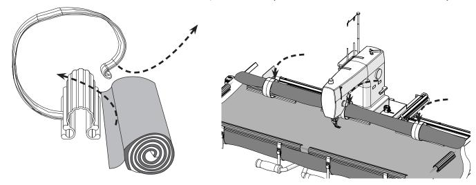
4 When it's time to move your fabric, remove the fabric roll from the coils. To remove the fabric clamps from the take-up rail, pry the lips of the clamp away from each other and then pull the clamp off the rail.
