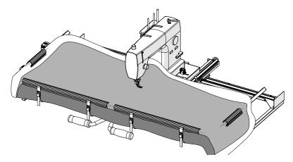
The coil clamps are much like how the original clamps on the Cutie frame worked. Press the coil clamps onto the take-up rail to hold the fabric in place. Make sure that the **end of the coil that is attached** to the clamp is on the inside of the frame.
