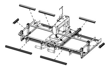
2 If you're using the coil clamps on the **take-up rail**, then remove the take-up rail from the frame by sliding open the two **take-up rail caps** on the sides of the frame, and then lifting the take-up rail up and guiding it through the machine throat. Otherwise, skip this step.
