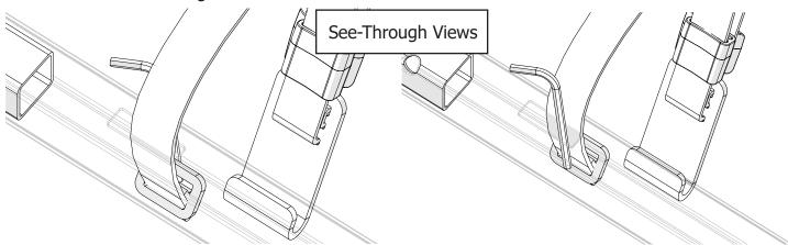
8 Once the metal holder is upright, line it up with the slot, using the Allen wrench to keep it upright, and pull the holder out of the rail.
