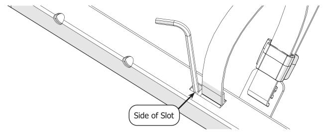
6 Use the Allen wrench to press the **metal holder** on the strap nearly to the bottom of the rail. Remember to only loosely hold the strap so that the metal holder can move freely.
