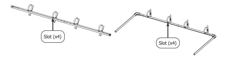
5 Pick a strap. While lightly holding the strap with one hand, use the other hand to insert the long end of the 2 mm Allen wrench into the **side of the slot**.
