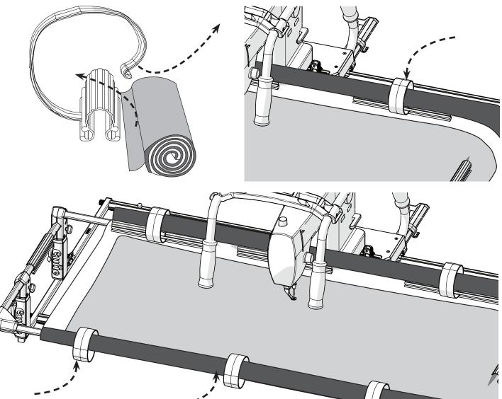
4 When it's time to move your fabric, if some of the quilt is in your coil clamps, then slide it out of the coils before you remove the clamps.
