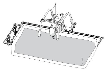
3 Press the coil clamps and the other clamps onto the rails to hold the fabric in place.
